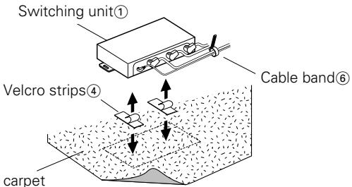
1. Remove the backing from the Velcro strips④ and attach it to the bottom of the switching unit①. Install the switching unit on the carpet.
