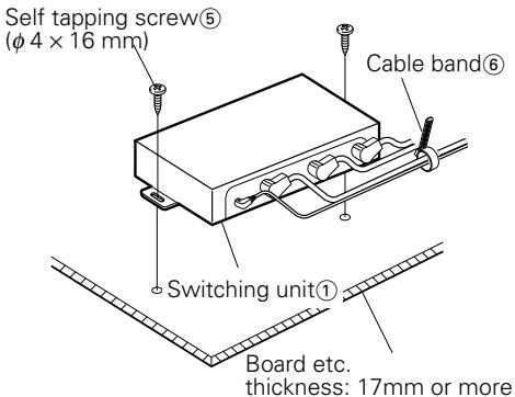
1. Install the switching unit with self-tapping screws⑤ ( $\phi 4 \times 16$  mm).
